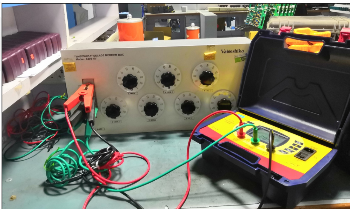
Calibration setup of a High Value Decade Resistance Box for Insulation Tester
