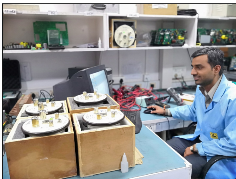
Calibration setup for Micro ohm Meter Calibration
