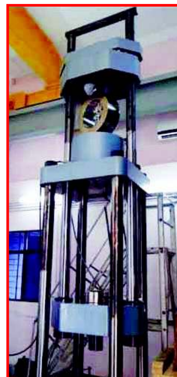
Vaiseshika successfully installed and commissioned 450 Ton Morehouse Load Cell Calibration Facility (having 0.025% accuracy) at the Satish Dhawan Space Centre, Sriharikota.
