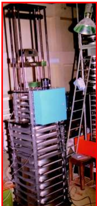
50 kN Dead Weight Calibrator (having 300 ppm uncertainty) at the National Physical Laboratory, New Delhi since 2001 as National Metrology Standard.
