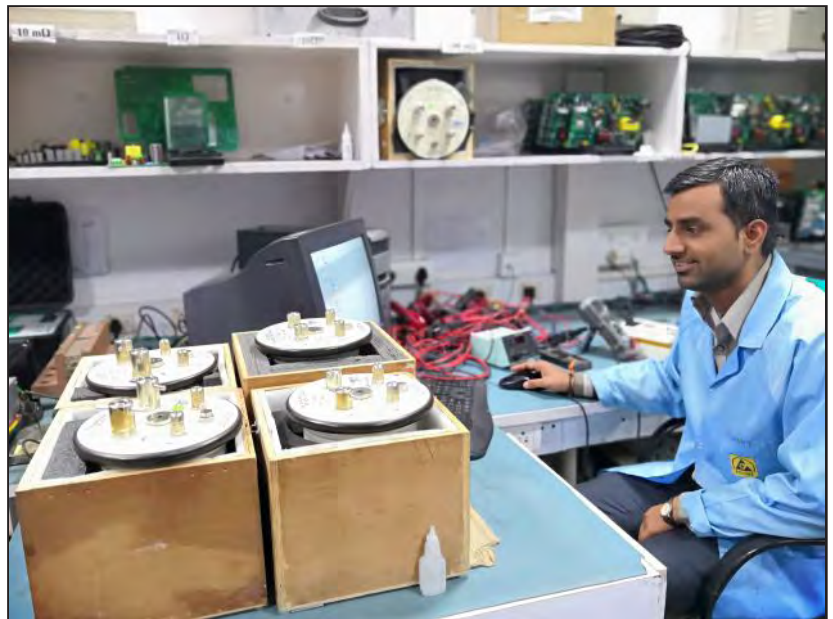
Calibration setup for Micro ohm Meter Calibration
