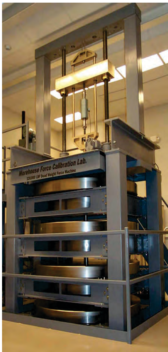
Morehouse Dead Weight Calibrator 1,20,000 lbf with CMC 0.0016% (Primary Force Calibration Reference Standard Installed at Morehouse Laboratory)
