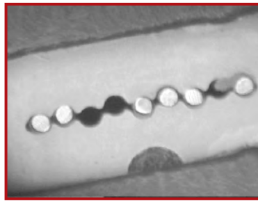
Printer head pins of a dot matrix printer (Black holes in the figure shows missing pins)
